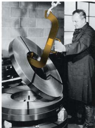
With the hook in place, the wedge pivots as the lift is started, and the coil begins to turn to a vertical position for transporting.
