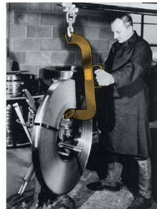
Coil being loaded on a stock reel. Hook is easily removed from the coil after releasing the hoist.
