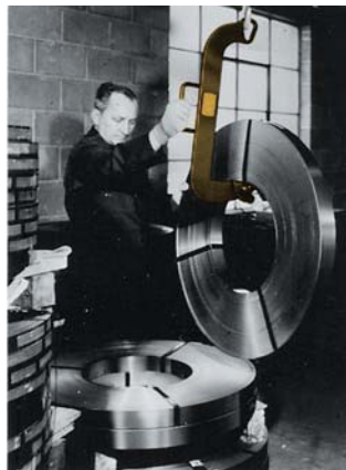
Coil is in vertical position after being lifted from its pallet. The weight of the coil holds the pivoting wedge in the vertical position during transportation.
