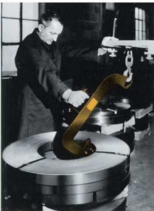
Placing spacer blocks between stacked coils permits easy insertion of the wedge. Lightweight and pivoting wedge makes it easy to position the hook.
